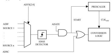
Using the ADC Interrupt Flag as a trigger source makes the ADC start a new conversion as soon as the ongoing conversion has finished. The ADC then operates in Free Running mode, constantly sampling and updating the ADC Data Register. The first conversion must be started by writing a '1' to ADCSRA.ADSC. In this mode the ADC will perform successive conversions independently of whether the ADC Interrupt Flag (ADIF) is cleared or not.
