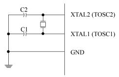
The Low Power Oscillator can operate in three different modes, each optimized for a specific frequency range. The operating mode is selected by the fuses CKSEL3...1, as shown in the following Table:
