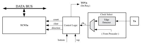
Depending of the mode of operation used, the counter is cleared, incremented, or decremented at each timer clock ( $clk_{T0}$ ).  $clk_{T0}$  can be generated from an external or internal clock source, selected by the Clock Select bits (CSO[2:0]). When no clock source is selected (CSO=0x0) the timer is stopped. However, the TCNT0 value can be accessed by the CPU, regardless of whether  $clk_{T0}$  is present or not. A CPU write overrides (has priority over) all counter clear or count operations.
