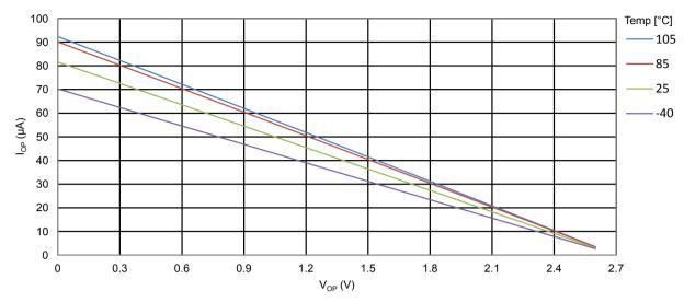
Figure 35-18 ATmega328PB: I/O Pin Pull-up Resistor Current vs. Input Voltage (V<sub>CC</sub> = 5V)
