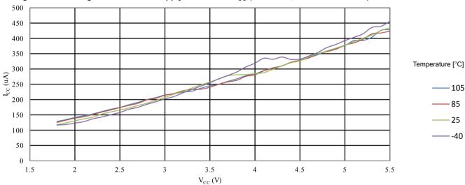
Figure 35-7 ATmega328PB: Active Supply Current vs. V<sub>CC</sub> (With ADC, No conversion)
