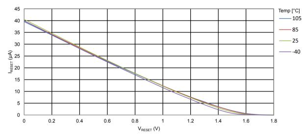
Figure 35-20 ATmega328PB: Reset Pull-up Resistor Current vs. Reset Pin Voltage  $(V_{CC} = 2.7V)$
