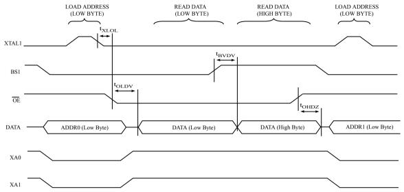
**Note:** The timing requirements shown in Parallel Programming Characteristics on page 386 (i.e.,  $t_{DVXH}$ ,  $t_{XHXL}$ , and  $t_{XLDX}$ ) also apply to reading operation.
