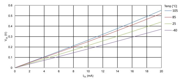
Figure 35-24 ATmega328PB: I/O Pin Output Voltage vs. Source Current (V<sub>CC</sub> = 3V)
