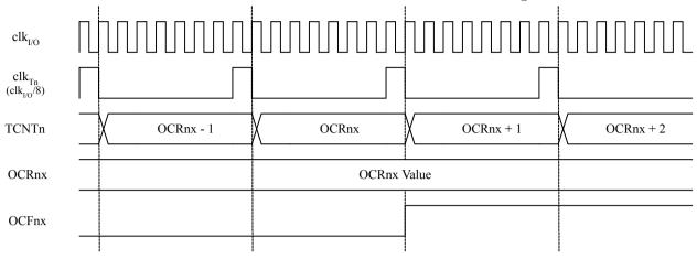
The next figure shows the setting of OCF0A and the clearing of TCNT0 in CTC mode and fast PWM mode where OCR0A is TOP.
