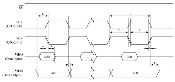
Figure 34-4 SPI Interface Timing Requirements (Slave Mode)
