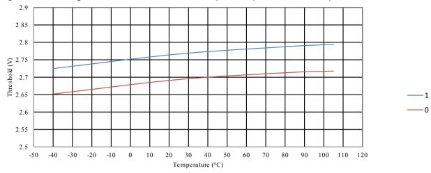
Figure 35-34 ATmega328PB: BOD Thresholds vs. Temperature (BODLEVEL is 4.3V)
