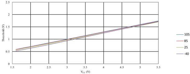
Figure 35-31 ATmega328PB Reset Pin Input Hysteresis vs. V<sub>CC</sub>
