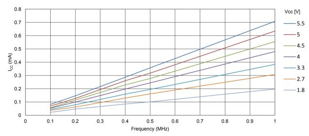
Figure 35-2 ATmega328PB: Active Supply Current vs. Frequency (1-20MHz)
