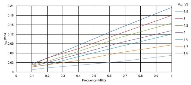
Figure 35-9 ATmega328PB: Idle Supply Current vs. Frequency (1-20MHz)
