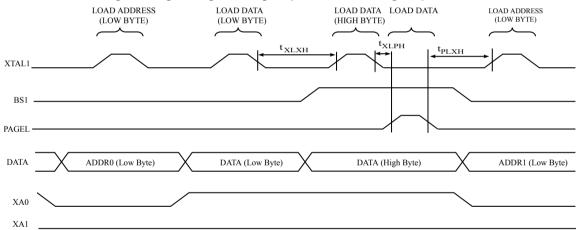
**Note:** The timing requirements shown in Parallel Programming Characteristics on page 386 (i.e.,  $t_{DVXH}$ ,  $t_{XHXL}$ , and  $t_{XLDX}$ ) also apply to loading operation
