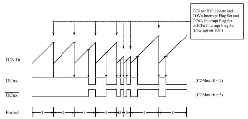
**Note:** The "n" in the register and bit names indicates the device number (n = 0 for Timer/Counter 0), and the "x" indicates Output Compare unit (A/B).
