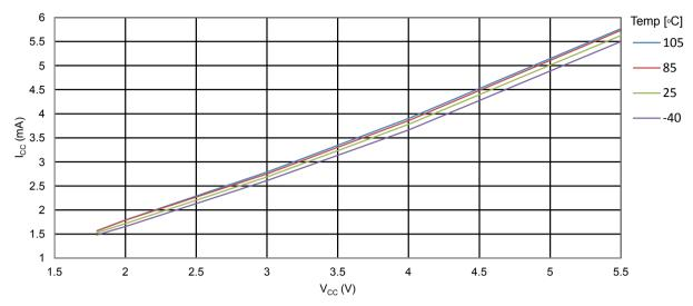
Figure 35-6 ATmega328PB: Active Supply Current vs. V<sub>CC</sub> (With ADC, conversion 50kHz)
