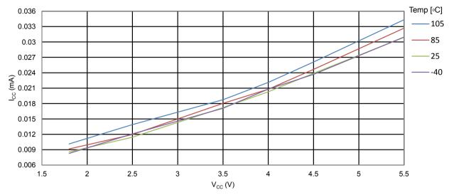
Figure 35-11 ATmega328PB: Idle Supply Current vs. V<sub>CC</sub> (Internal RC Oscillator, 1MHz)
