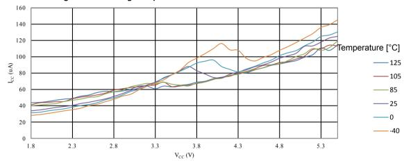
Figure 35-49 ATmega328PB: AREF External Reference Current vs. Vcc
