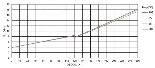
Figure 35-46 ATmega328PB: OSCCAL Value StepSize in %. Base Frequency = 8.0MHz
