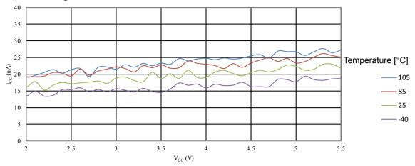
Figure 35-51 ATmega328PB: Programming Current vs. Vcc
