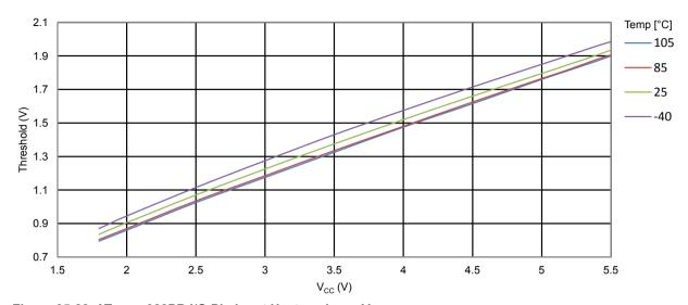
Figure 35-28 ATmega328PB I/O Pin Input Hysteresis vs. V<sub>CC</sub>
