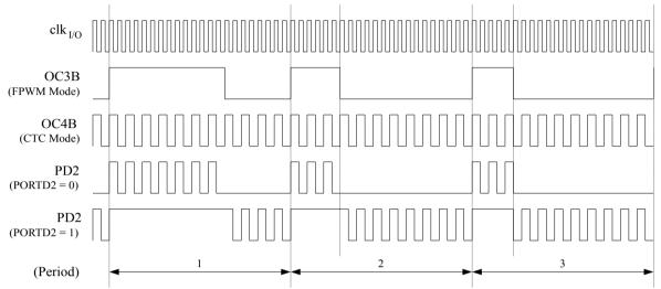
In this example, Timer/Counter4 provides the carrier, while the modulating signal is generated by the Output Compare unit B of the Timer/Counter3.
