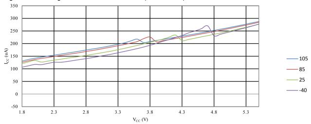
Figure 35-48 ATmega328PB: Analog Comparator Current vs. Vcc
