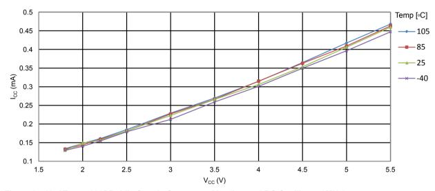
Figure 35-12 ATmega328PB: Idle Supply Current vs. V<sub>CC</sub> (Internal RC Oscillator, 8MHz)
