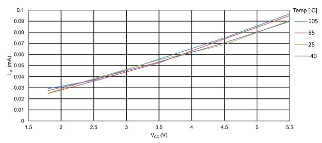
Figure 35-4 ATmega328PB: Active Supply Current vs. V<sub>CC</sub> (Internal RC Oscillator, 1MHz)
