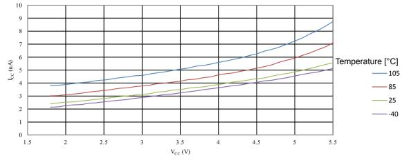
Figure 35-15 ATmega328PB: Power-Down Supply Current vs. V<sub>CC</sub> (AREF, VCCDIV2)
