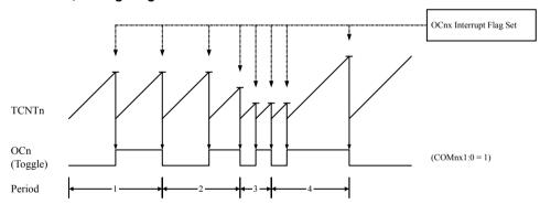
An interrupt can be generated each time the counter value reaches the TOP value by setting the OCF0A Flag. If the interrupt is enabled, the interrupt handler routine can be used for updating the TOP value.
