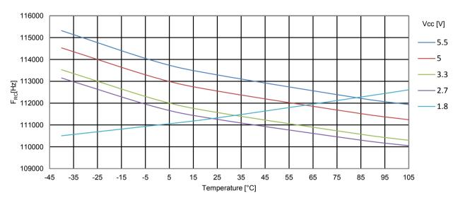
Figure 35-42 ATmega328PB: Watchdog Oscillator Frequency vs. V<sub>CC</sub>
