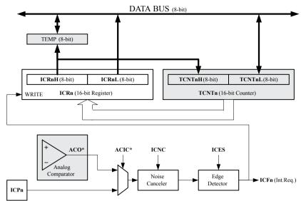
**Note:** Analog comparator can be used for only Timer/Counter1 and not applicable for Timer/Counter3 or Timer/Counter4.
