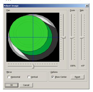
The various sliders can be used to pan, zoom and spin the image, while the checkboxes can be used to mirror it horizontally or vertically. The Show Center checkbox shows or hides the blue lines that mark the center of the image, while the Reset button can be used to restore the image to its original state. The various manipulation options are typically used to modify an image in order to create various different states for use in animation.
