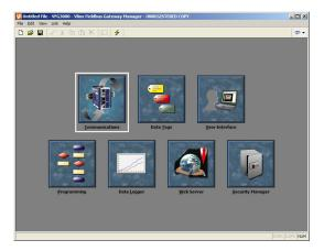
The software is designed such that the first three icons are the only ones required for the majority of simple applications. The remainder of the icons provide access to the Gateway's more advanced features, such as programming, data logging and the Gateway's web server.
