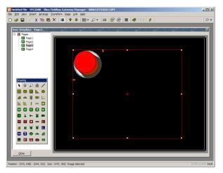
The now-reduced image can be moved within the whole primitive by defining values to control its horizontal and vertical position. These values are defined together with minimum and maximum limits that specify the values corresponding to the extremes of the image's movement within the primitive's bounding rectangle...
