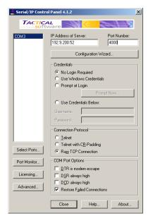
You will now be able to configure any Windows-based software to use the newly-created COM port for download. When the software opens the connection, the Gateway will suspend communications on the shared port, and then data will be exchanged between the PC software and the remote PLC—just as if they were connected directly! When the port is closed, or if no data is transferred for a minute, communications will be resumed.
