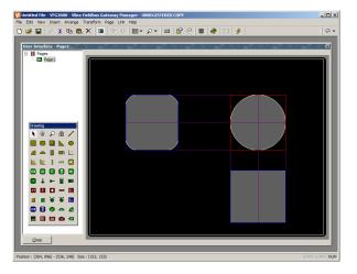
Guidelines are present at both the edges of the figures, and at the center, showing that both the edges and the centers are aligned. The red rectangle is highlighting the newly-created primitive, while the blue rectangles are highlighting the primitives to which the guidelines have been drawn. Smart Align is also enabled when primitives are moved or re-sized.
