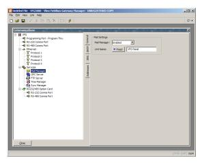
The properties on a General tab are used to enable or disable mail manager, and to provide a name for the Fieldbus Gateway. This name will be used within email messages to identify the originator of the message. Applications will typically use the name of the machine to which the Gateway is attached, or the name of the site that it is monitoring.
