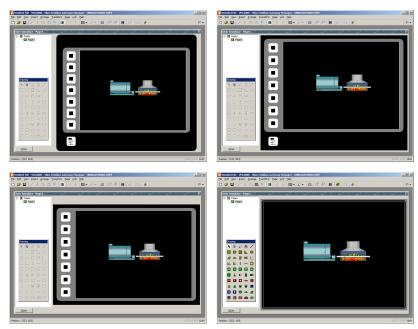
As you can see, at each level, fewer keys are shown, and more of the window is allocated to the display itself. The view level can be controlled from the View > Panel menu, or by using the panel icon  $\square$ , or by pressing the Alt key together with the digits 1 through 4.
