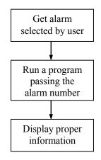
The first step is achieved using the system variable **Data**. This system variable is only available for the OnHelp field and contains information on the alarm selected. **Data** is a Long (Double word) and contains the following information:
