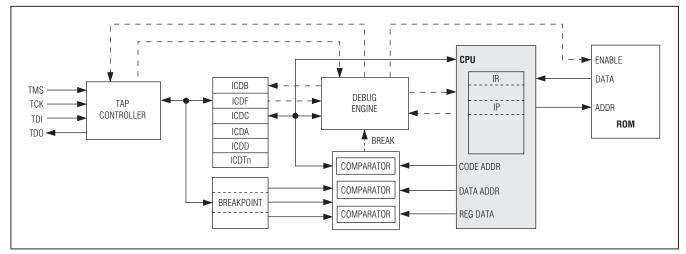
Figure 12-1. In-Circuit Debugger
