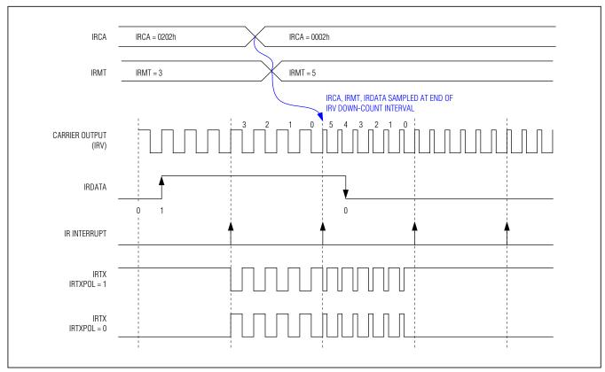
Figure 8-1. IR Transmit Frequency Shifting Example (IRCFME = 0)
