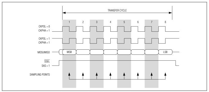
Figure 10-2. SPI Transfer Formats (CKPHA = 1)
