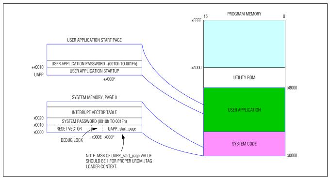
Figure 2-8. Program Memory Segmentation (Only Two Segments)
