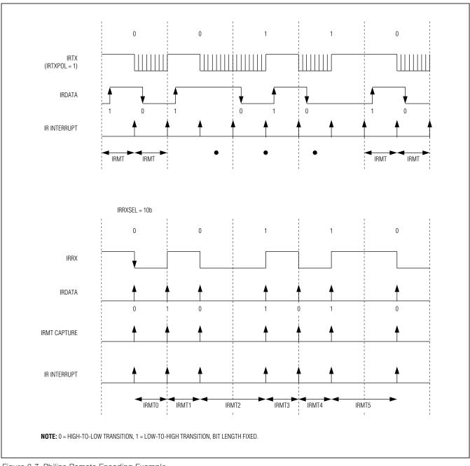
Figure 8-7. Philips Remote Encoding Example
