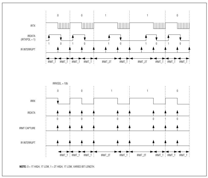
Figure 8-8. Sony Remote Encoding Example
