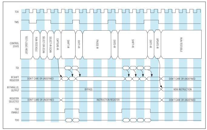
Figure 11-3. TAP Controller Debug Mode IR-Scan Example
