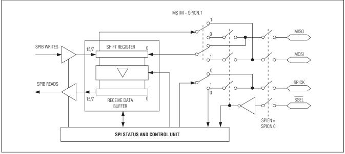
Figure 10-1. SPI Block Diagram
