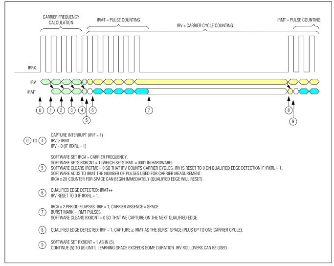
Figure 8-6. Receive Burst-Count Example
