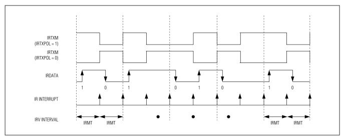
Figure 8-4. External IRTXM (Modulator) Output
