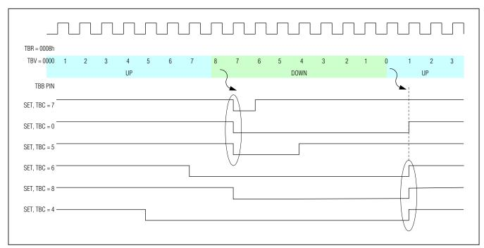
Figure 7-6. Timer B PWM Output Up/Down-Count Examples
