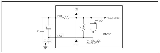
Figure 2-10. On-Chip Crystal Oscillator
