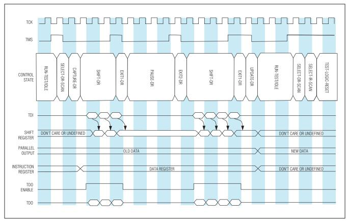
Figure 11-4. TAP Controller Debug Mode DR-Scan Example
