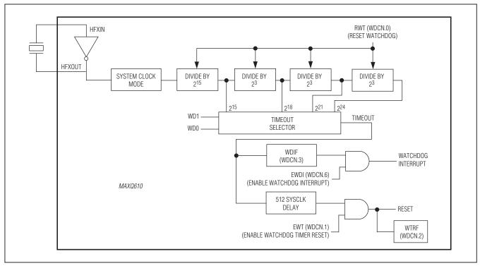
Figure 3-1. Watchdog Timer Block Diagram
