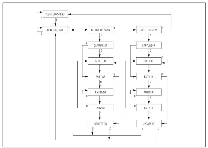
Figure 11-1. TAP Controller State Diagram
