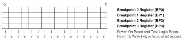
These registers are accessible only through background mode read/write commands. These four registers serve as program memory address breakpoints. When DME bit is set in background mode, the debug engine monitors the program address bus activity while the CPU is executing the user program. If an address match is detected, a break occurs, allowing the debug engine to take control of the CPU and enter debug mode.
