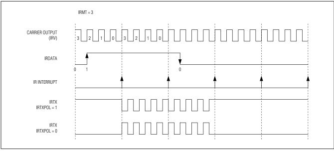
Figure 8-3. IR Transmission Waveform (IRCFME = 0)
