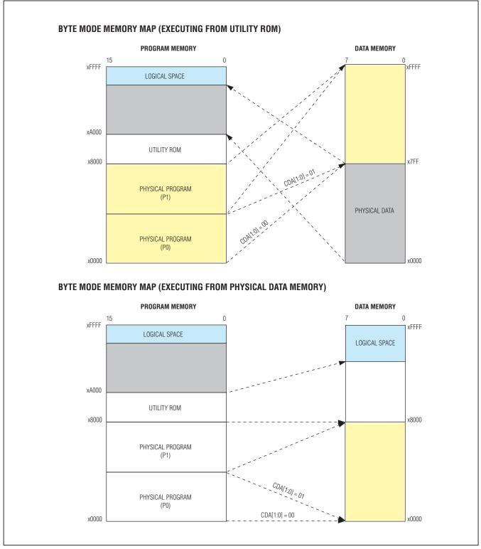
Figure 2-5. CDA Functions in Byte Mode
