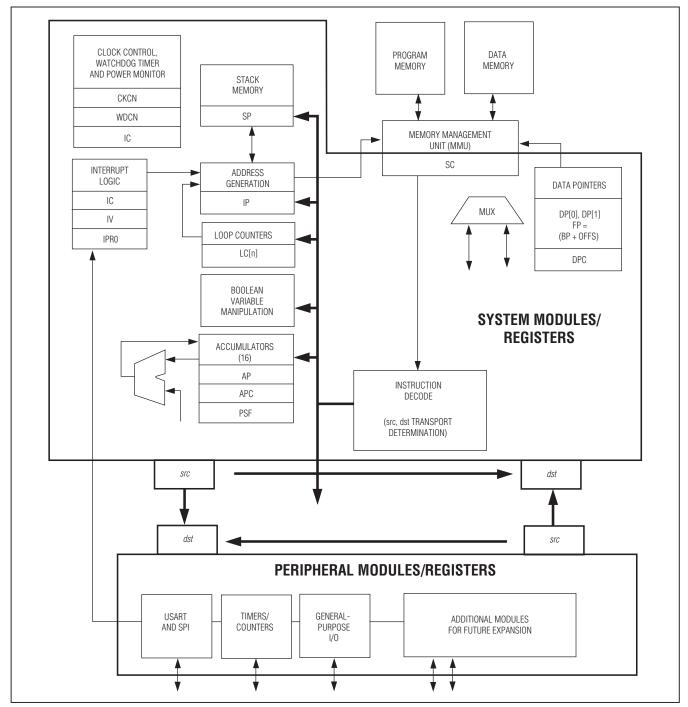
Figure 2-1. MAXQ610 Transport-Triggered Architecture
