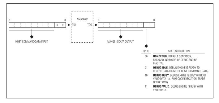
The data byte portion of the 10-bit shift register is interfaced directly to the ICDB parallel register. The ICDB register functions as the holding data register for both transmit and receive operations. On the falling edge of TCK in the update-DR state, the outgoing data is loaded from the ICDB parallel register to the debug shift register and the incoming shift register data is latched in the ICDB parallel register.
