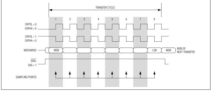
Figure 10-3. SPI Transfer Formats (CKPHA = 0)
