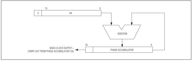
Figure 9-5. Baud-Clock Generator
