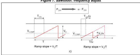
Figure 7. Sawtooth: frequency adjust
