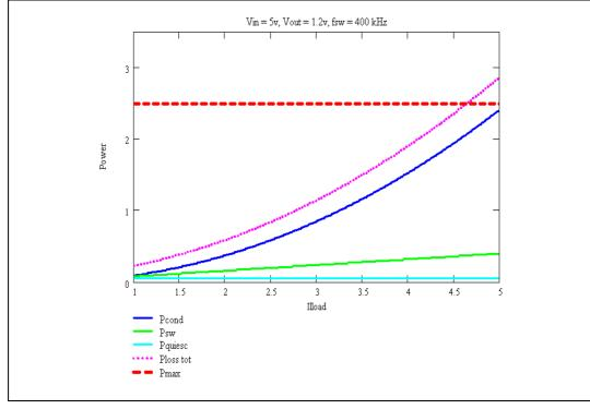
Figure 21. Estimation of the internal power losses
