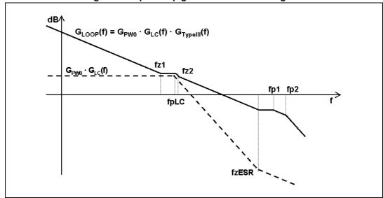
Figure 13. Open loop gain: module bode diagram
