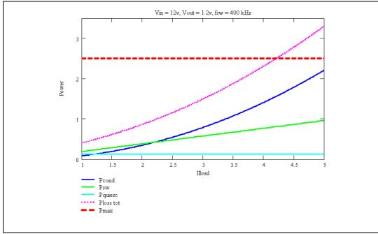
Figure 20. Estimation of the internal power losses
