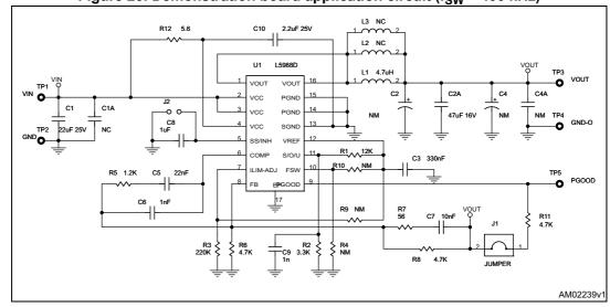
Figure 25. Demonstration board application circuit (f<sub>SW</sub> = 400 kHz)
