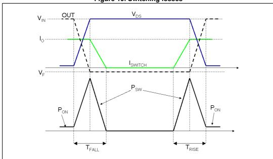
Figure 19. Switching losses
