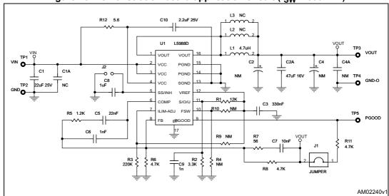
Figure 26. Demonstration board application circuit ( $f_{SW}$  = 600 kHz)
