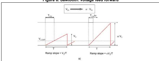
Figure 6. Sawtooth: voltage feed forward
