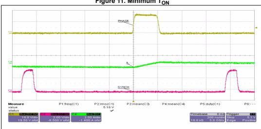
Figure 11. Minimum T<sub>ON</sub>
