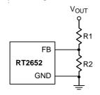
Figure 1. Setting the Output Voltage
