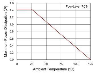
Figure 2. Derating Curve of Maximum Power Dissipation
