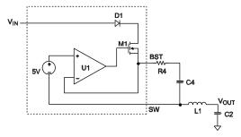
Figure 3: Internal Bootstrap Charging Circuit
