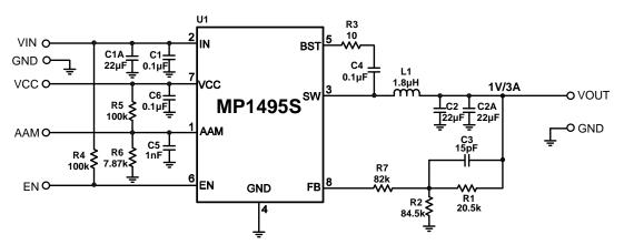
Figure 12: 12V<sub>IN</sub>, 1V/3A Output
