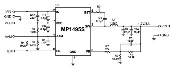
**Figure 11: 12V<sub>IN</sub>, 1.2V/3A Output**
