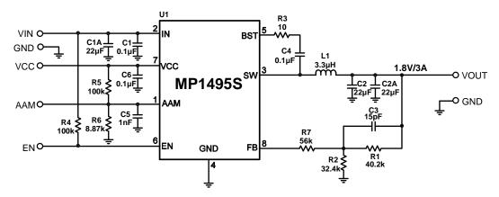
**Figure 10: 12V<sub>IN</sub>, 1.8V/3A Output**
