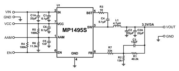
Figure 8: 12V<sub>IN</sub>, 3.3V/3A Output
