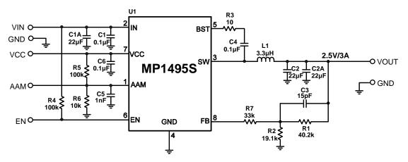
Figure 9: 12V<sub>IN</sub>, 2.5V/3A Output
