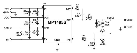
Figure 7: 12V<sub>IN</sub>, 5V/3A Output
