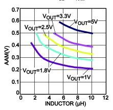
Figure 6: AAM Selection for Common Output Voltages (V<sub>IN</sub>=4.5V to 16V)
