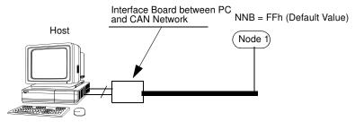
Figure 7. On Network Connection
