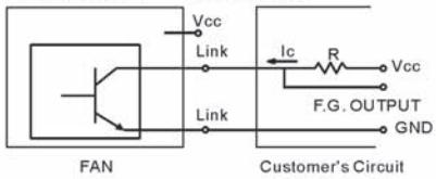
Vcc=From + 5 To +28 VDC      Do not exceed fan supply voltage
