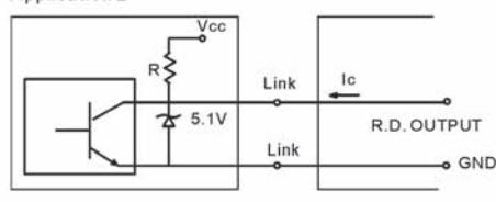
Vcc= From + 5 To +28 VDC ( Generally using + 12 or + 24VDC )
