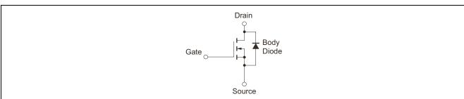
Remark: Strong electric field, when exposed to this device, can cause destruction of the gate oxide and ultimately degrade the device operation. Steps must be taken to stop generation of static electricity as much as possible, and quickly dissipate it once, when it has occurred.
