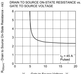
V<sub>GS</sub> - Gate to Source Voltage - V
