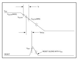
**FIGURE 3-4:** Timing Diagram – Power Down (TC1277).
