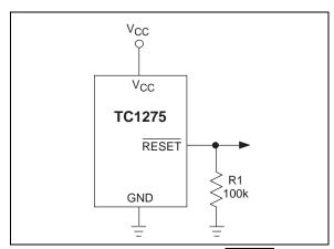
**FIGURE 3-6:** ENSURING RESET VALID TO  $V_{CC} = 0V$ .
