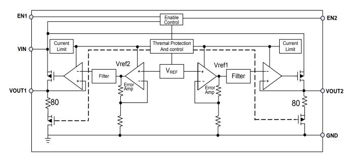
Figure 1—Function Block Diagram
