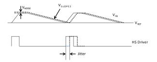
Figure 5—Jitter in Skip Mode
