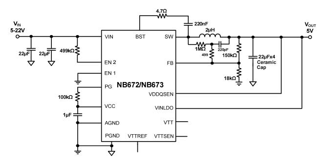
Figure 16 – Typical Application Circuit with Low ESR Ceramic Output Capacitor V<sub>IN</sub>=7-22V, V<sub>OUT</sub>=5V
