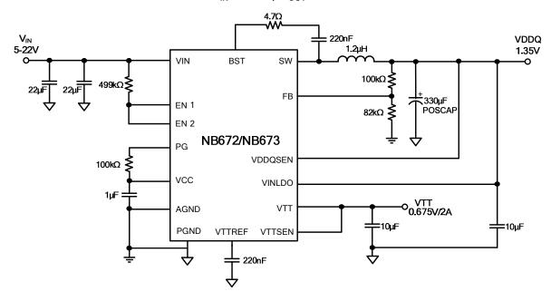
Figure 15 — Typical Application Circuit with Large ESR POSCAP Output Capacitor  $V_{\text{IN}}$ =5-22V,  $V_{\text{OUT}}$ =1.35V
