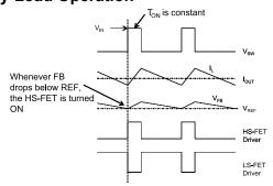
Figure 2—Heavy Load Operation
