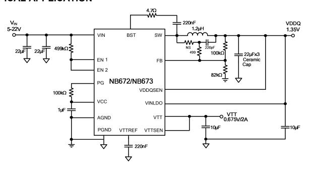
Figure 14 — Typical Application Circuit with Low ESR Ceramic Output Capacitor  $V_{IN}$ =5-22V,  $V_{OUT}$ =1.35V
