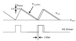
Figure 4—Jitter in PWM Mode
