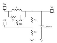
Figure11—Simplified Circuit of Ceramic Capacitor
