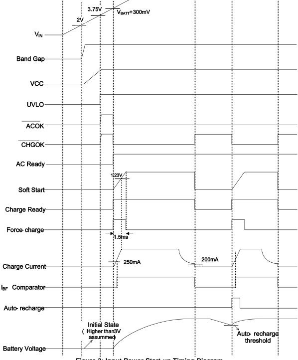
Figure 3: Input Power Start-up Timing Diagram
