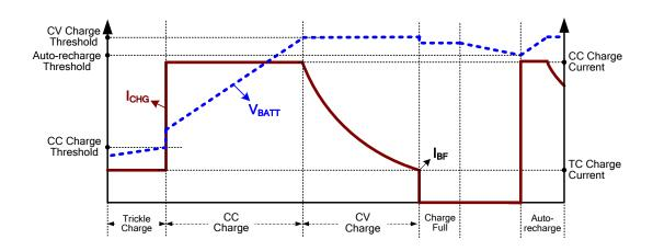
Figure 2: Li-ion Battery Charge Profile
