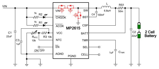
Figure 7: Typical Application Circuit to Charge a 2 Cell Battery with 12V<sub>IN</sub>.
