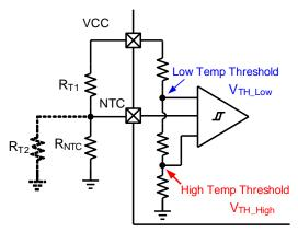
Figure 5: NTC Function Block
