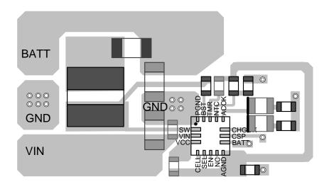
Figure 6: MP2615 PCB Guild Design
