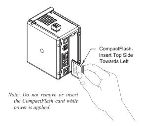
Information stored on a CompactFlash card can be read by a card reader attached to a PC. This information is stored in IBM (Windows®) PC compatible FAT16 file format.
