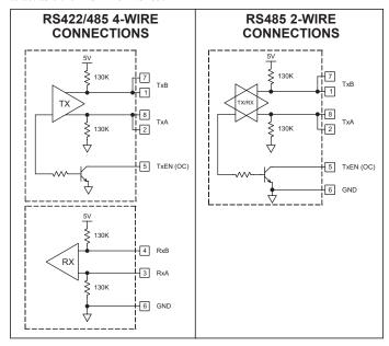
Note: All B&B devices connect A to A and B to B.
