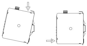
Figure 1 - Attach Fieldbus Gateway To DIN Rail
