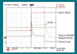
M-FIAM7 output response to an input transient.
