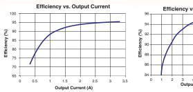
PRM Efficiency vs. Output Current
