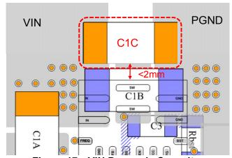
Figure 17—VIN Decouple Capacitor
