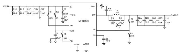
Figure 14 — Typical Application Circuit with Low ESR Ceramic Capacitor MPQ8616, V<sub>IN</sub>=5V, V<sub>OUT</sub>=1.2V, I<sub>OUT</sub>=6/12A, f<sub>SW</sub>=600kHz
