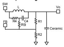
Figure8—Simplified Circuit of Ceramic Capacitor
