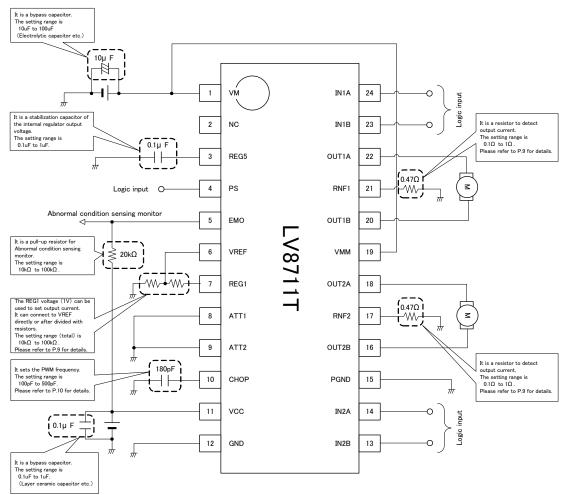
Figure 29. Typical application Circuit for DC motors
