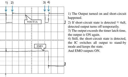
Figure 26. Timing chart of the Output short-circuit protection and EMO
