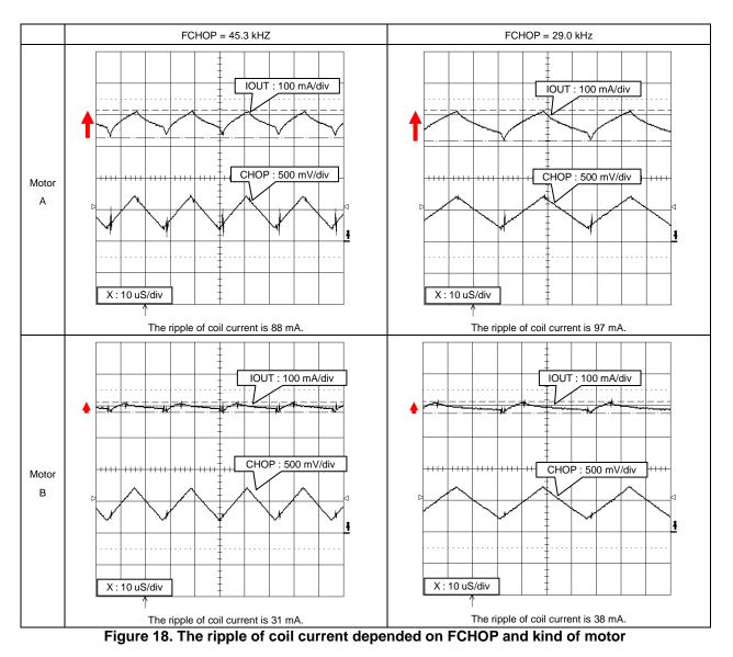
The ripple of coil current depends on coil impedance or coil inductance of motor. The ripple is different even if chopping frequency is set the same value.
