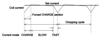
The IC switches to SLOW DECAY after Blanking section, and then switches to FAST DECAY mode for the last  $1\mu$ s.
