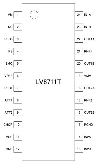
Figure 1. Pin Assignment
