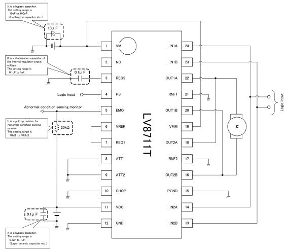
Figure 30. Typical application Circuit for 1 DC motor
