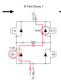
4)After Slow Decay 2, Tr\_BD turns OFF. The coil current flow through RF, Tr\_AD, coil and Di\_BU to VMM. At that time, output voltages are  $OUT\_A: 0V + Vsat + I \times RF$ (Negative potential)
