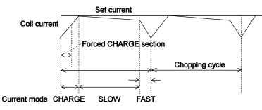
Charge mode continues until  $I_{COIL} \ge I_{REF}$ . After the IC switches to SLOW DECAY mode and then switches to FAST DECAY mode for the last 1 $\mu$ s.
