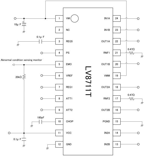
Figure 32. Evaluation Board circuit schematic
