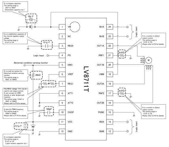
Figure 28. Typical application Circuit for Stepping motor
