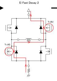
5)If Di\_BU keeps to flow current, the IC chip generate heat. Then Tr\_BU turns ON in Fast Decay 2.
