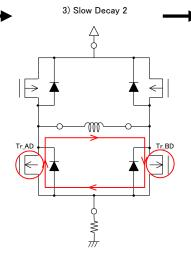
3)If Di\_AD keeps to flow current, the IC chip generates heat. Then Tr\_AD turns ON in Slow Decay 2. At that time, output voltages are
