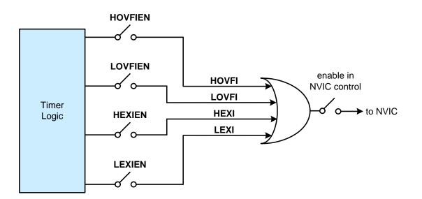
Figure 36.4. Timer Interrupt Configuration
