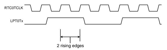
Figure 30.2. External Input Clock Synchronization Timing
