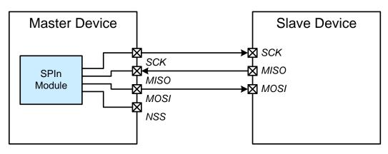
Figure 35.5. 3-Wire Single Master Mode Connection Diagram
