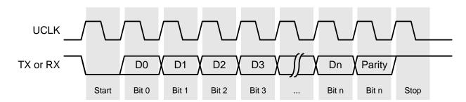
Figure 37.4. Synchronous Communication
