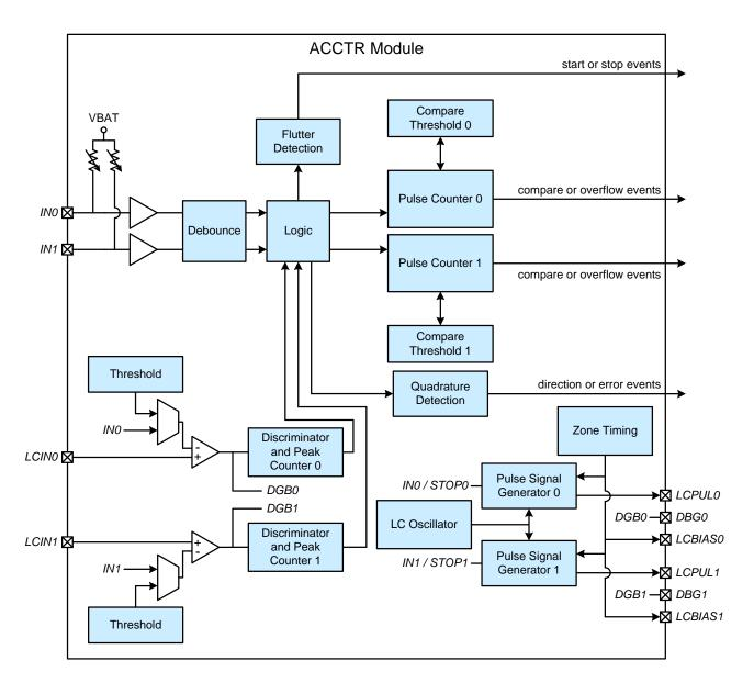
Figure 14.1. ACCTR Block Diagram
