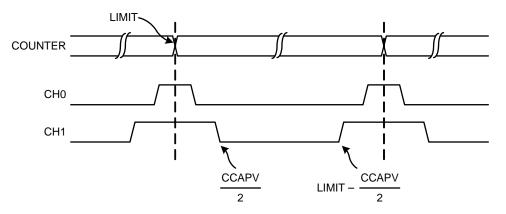
Figure 22.7. Multiple Center-Aligned PWM Channels
