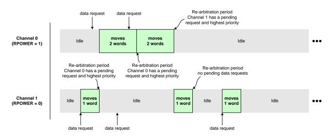
Figure 17.7. DMA Arbitration Example
