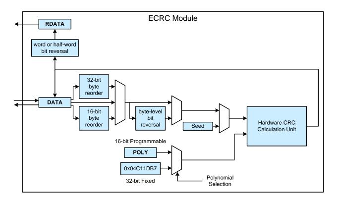
Figure 20.1. ECRC0 Block Diagram
