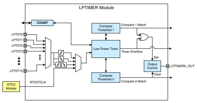
Figure 30.1. Low Power Timer Block Diagram
