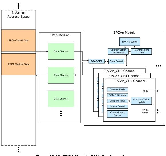
Figure 22.15. EPCA Module DMA Configuration
