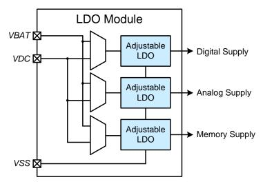
Figure 11.1. LDO0 Block Diagram
