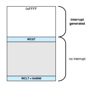
Figure 34.12. Example Window Comparator Limits for Above Value (WCGT = Value, WCLT = 0)
