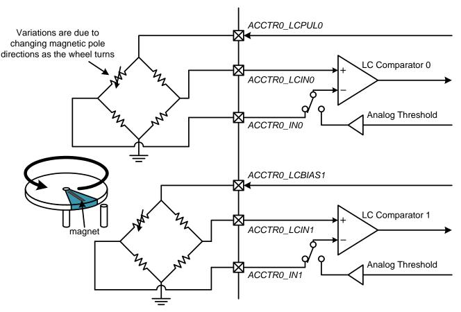
Figure 14.4. Wheatstone Bridge Configuration
