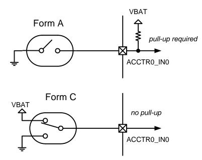
Figure 14.2. Reed Switch Configurations
