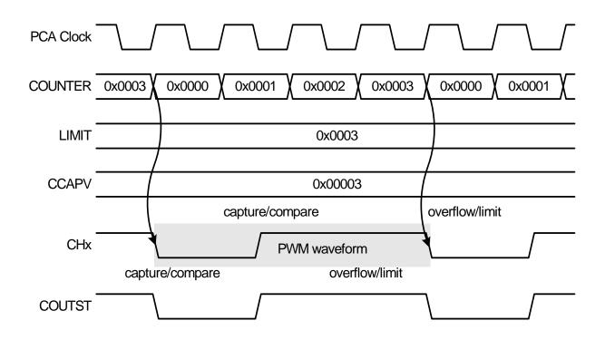
Figure 22.6. Example Edge-Aligned PWM Timing Diagram
