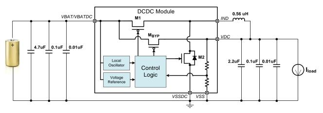
Figure 12.1. DCDC0 Block Diagram
