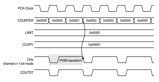
Figure 22.13. Example N-bit Edge-Aligned PWM Timing Diagram
