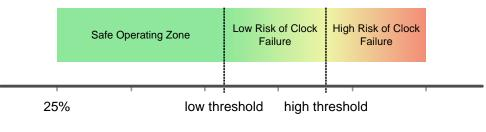
RTCn Oscillator (RTCnOSC) Duty Cycle
