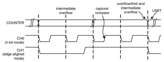
Figure 22.12. Multiple Edge-Aligned PWM Channels (N-bit and Edge-Aligned)
