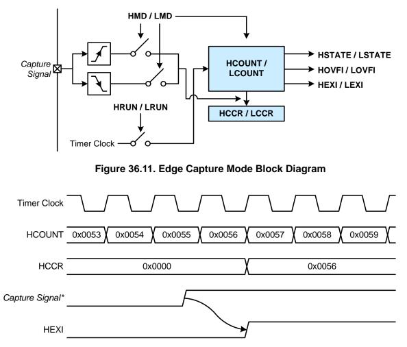
\*Note: The timer response delay to capture input signal changes is 3-4 APB clock cycles.
