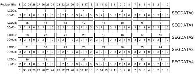
Figure 27.2. LCD Data Register to LCD Pin Mapping
