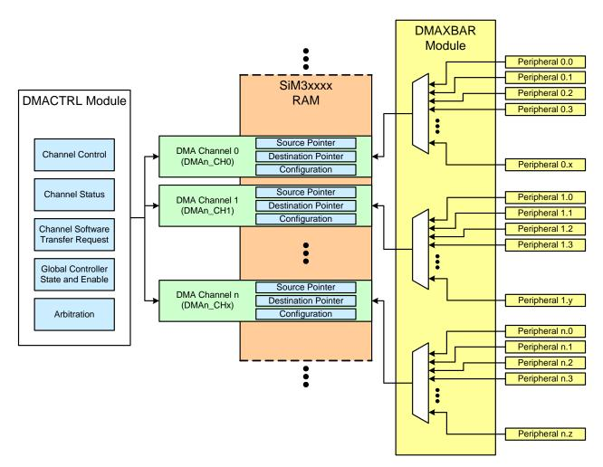
Figure 17.1. DMACTRL and DMACH Block Diagram
