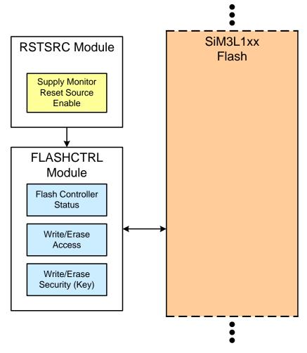
Figure 24.1. Flash Controller Block Diagram
