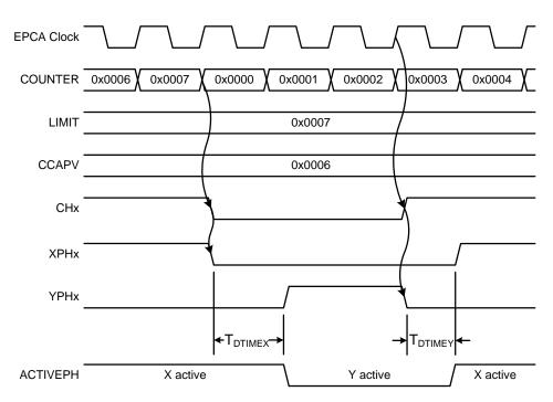
Figure 22.4. Example Channel Differential Output Timing Diagram
