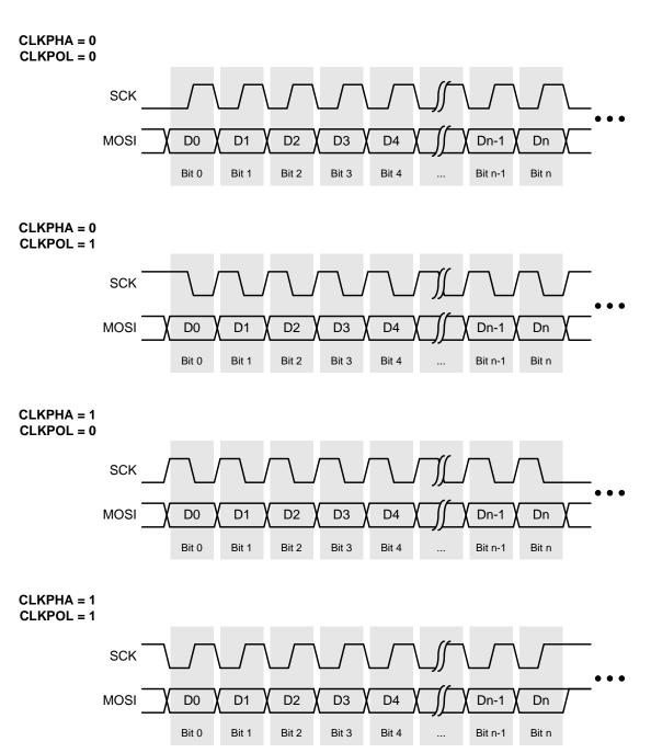
Figure 35.4. SPI Clock Polarity and Phase Combinations (DDIRSEL = 1, Master Mode)
