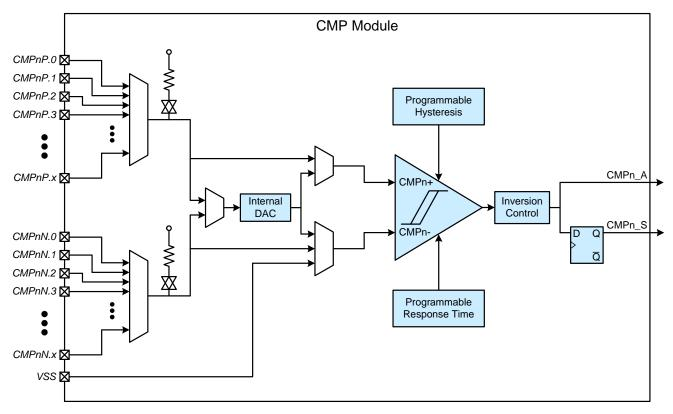
Figure 16.1. Comparator Block Diagram
