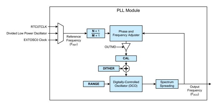
Figure 31.1. PLL Block Diagram
