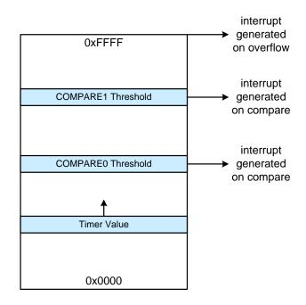
Figure 30.3. Low Power Timer Operation
