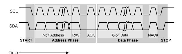
Figure 25.3. Typical I2C 7-bit Address Transaction
