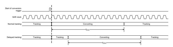
Figure 34.3. Non-Burst Tracking and Conversion Timing
