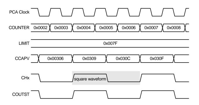
Figure 22.10. Example High-Frequency Square Wave Mode Timing Diagram
