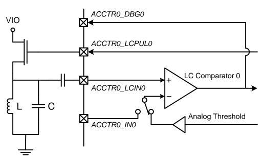
Figure 14.3. LC Resonant Configuration
