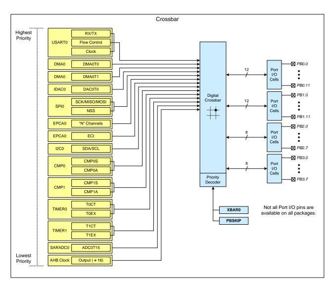
Figure 8.1. Crossbar 0 Block Diagram
