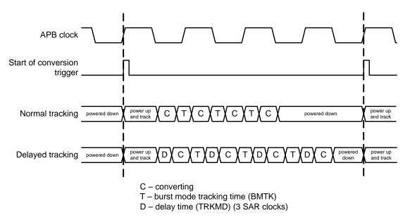
Figure 34.5. Burst Mode Tracking and Conversion Timing (Four Samples)
