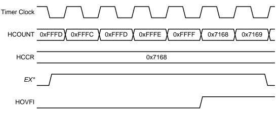
\*Note: The timer response delay to EX input signal changes is 3-4 APB clock cycles.
