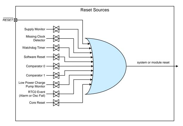
Figure 7.1. Reset Sources Block Diagram
