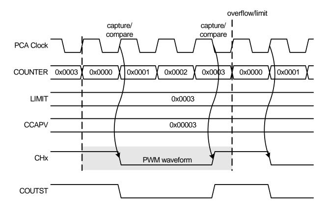
Figure 22.8. Example Center-Aligned PWM Timing Diagram
