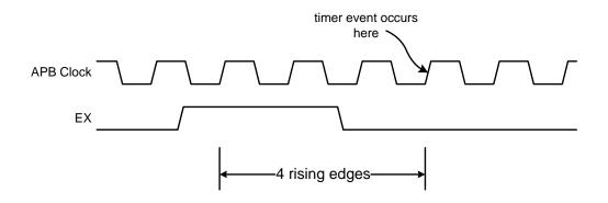
Figure 36.6. EX Signal Synchronization Timing
