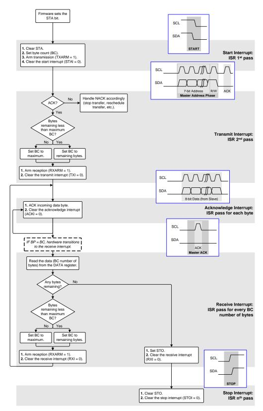
Figure 25.9. Master Read Flow Diagram (7-bit Address)
