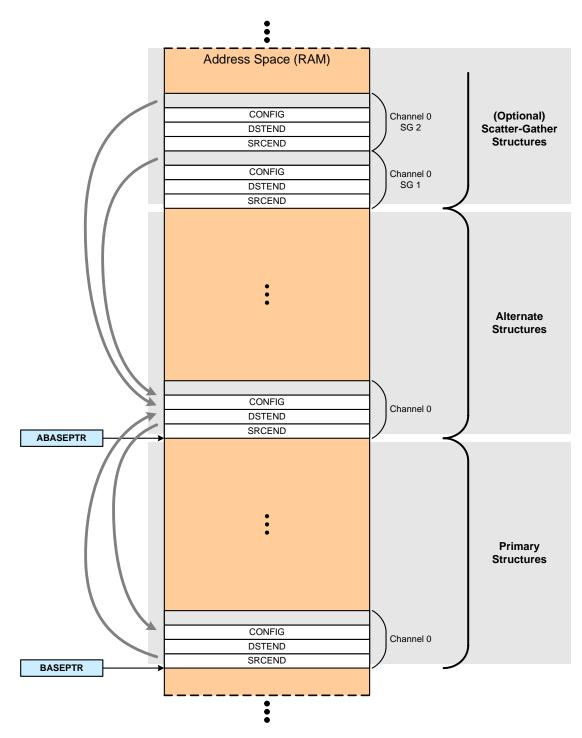
Figure 17.6. Memory and Peripheral Scatter-Gather Transfer Memory Configuration
