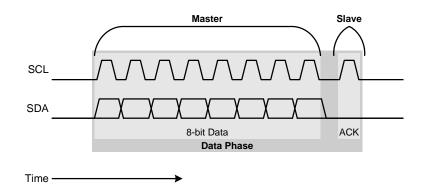
Figure 25.7. Single Byte I2C Write Data Phase
