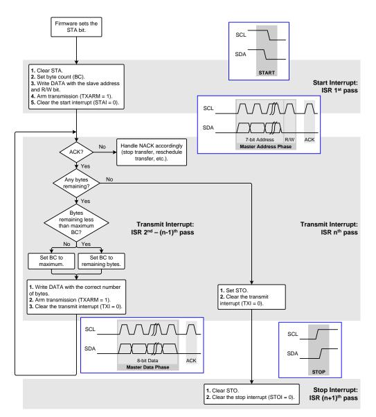
Figure 25.8. Master Write Flow Diagram (7-bit Address)
