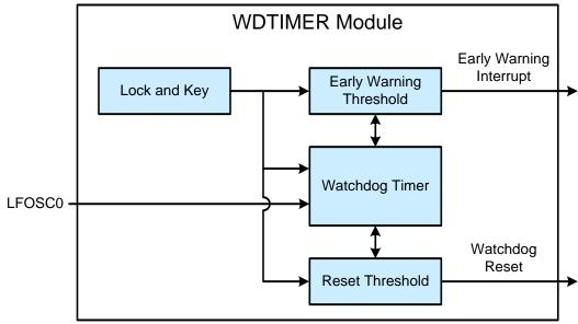
Figure 41.1. Watchdog Timer Block Diagram
