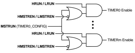
Figure 36.5. Timer Synchronization Block Diagram
