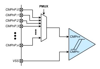
Figure 16.3. Comparator Input Mode 1 (INMUX = 1)
