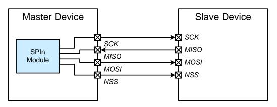
Figure 35.6. 4-Wire Single Master Mode Connection Diagram
