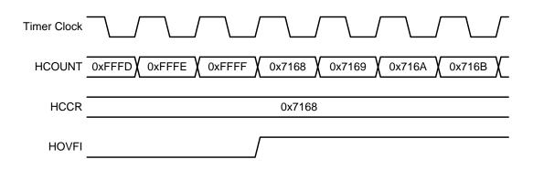
Figure 36.8. 16-bit Auto-Reload Mode Timing Diagram
