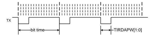
Figure 37.6. Transmit IrDA Pulse Width Timing
