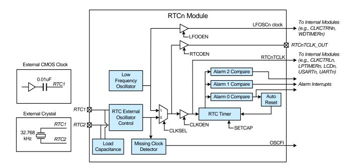
Figure 33.1. RTC Block Diagram
