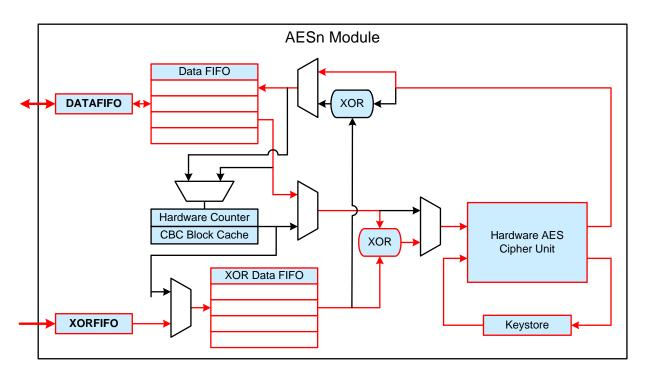
Figure 15.8. Cipher Block Chaining (CBC) AES Module Block Diagram—Encryption
