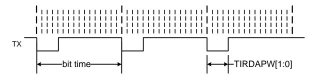
Figure 38.4. UART Transmit IrDA Pulse Width Timing
