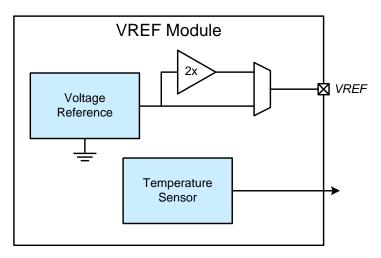
Figure 40.1. Voltage Reference Block Diagram
