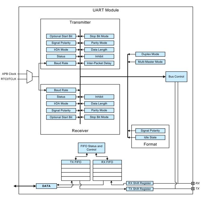
Figure 38.1. UART Block Diagram
