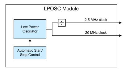
Figure 29.1. Low Power Oscillator Block Diagram
