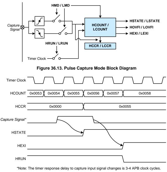
Figure 36.14. Pulse Capture Mode Timing Diagram (High Pulse Shown)
