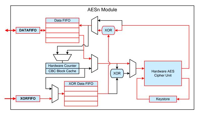
Figure 15.9. Cipher Block Chaining (CBC) AES Module Block Diagram—Decryption
