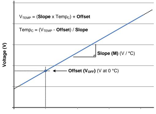
Temperature (°C) Figure 40.2. Temperature Sensor Transfer Function
