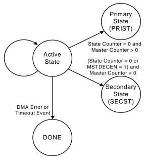
Figure 19.2. State Transition Diagram
