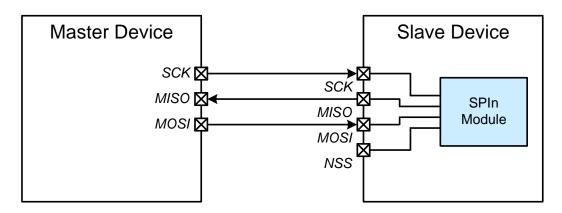
Figure 35.9. 3-Wire Single Slave Mode Connection Diagram
