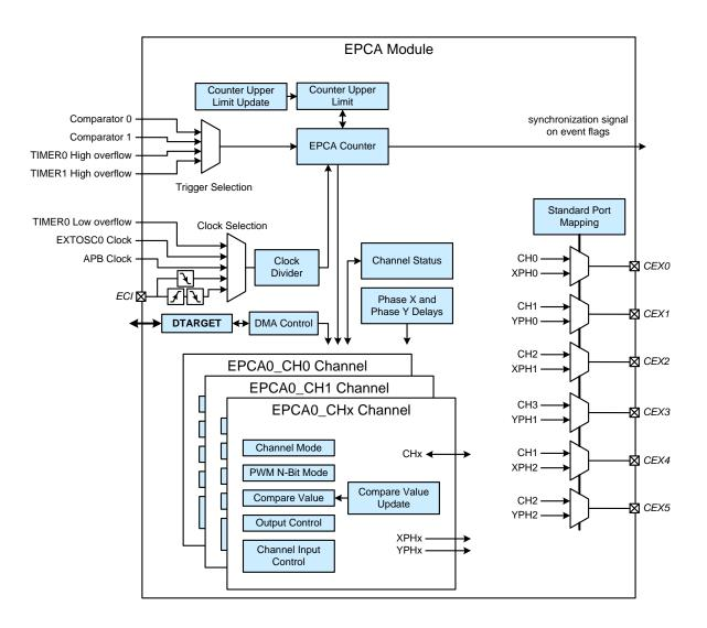
Figure 22.1. EPCA Block Diagram
