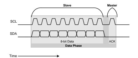
Figure 25.6. Single Byte I2C Read Data Phase
