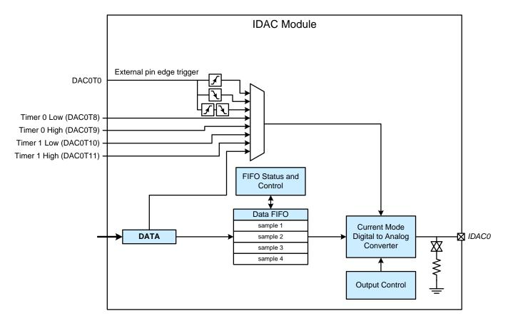
Figure 26.1. IDAC Block Diagram
