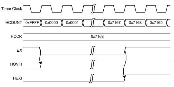
Figure 36.22. PWM Mode Timing Diagram
