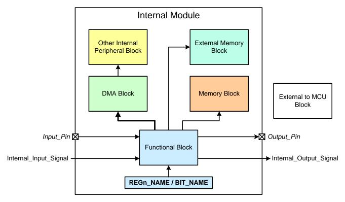
Figure 1.1. Block Diagram Conventions
