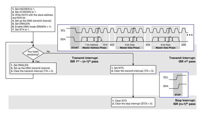
Figure 25.17. Master Write with DMA and Automatic Hardware Flow Diagram (7-bit Address)
