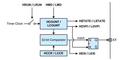
Figure 36.21. PWM Mode Block Diagram
