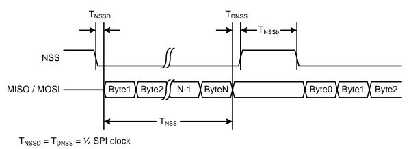
$T_{NSS} = NSSCNT+1$  Bytes
