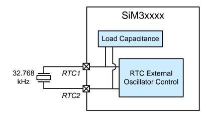
Figure 33.2. Crystal Mode Hardware Configuration
