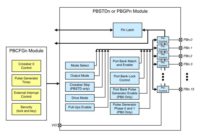
Figure 8.3. PBSTD and PBGP Block Diagram
