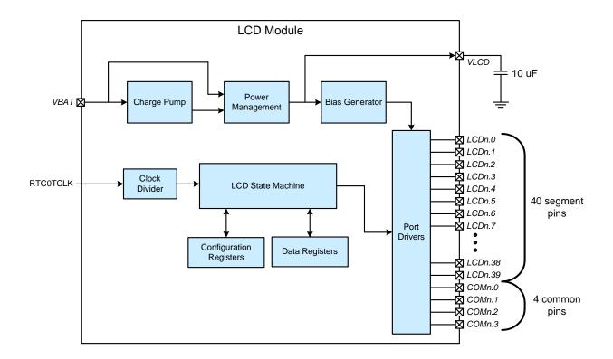
Figure 27.1. LCD0 Block Diagram
