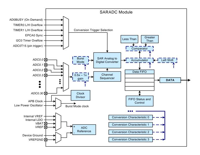
Figure 34.1. SARADC Block Diagram
