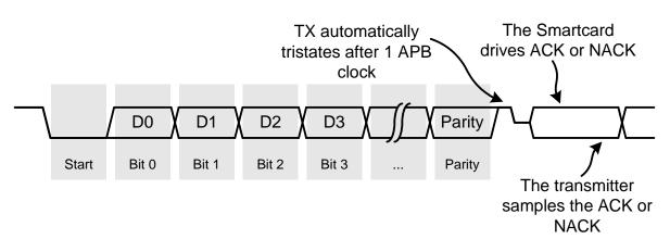
Figure 37.7. Smartcard Transmit Signalling
