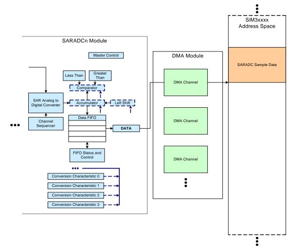
Figure 34.14. SARADC DMA Configuration
