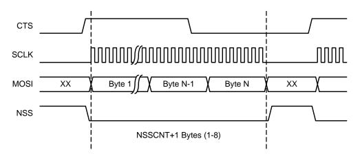
Figure 35.13. Transmit On Request Mode Timing
