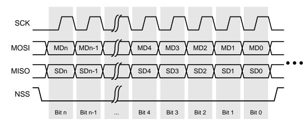
Figure 35.2. 4-Wire SPI Transfer
