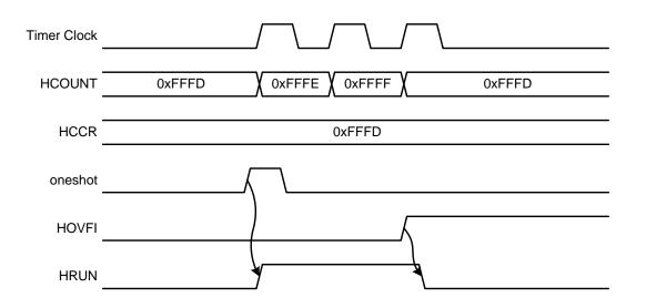
Figure 36.18. One Shot Mode Timing Diagram
