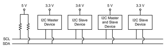
Figure 25.2. I2C Hardware Configuration
