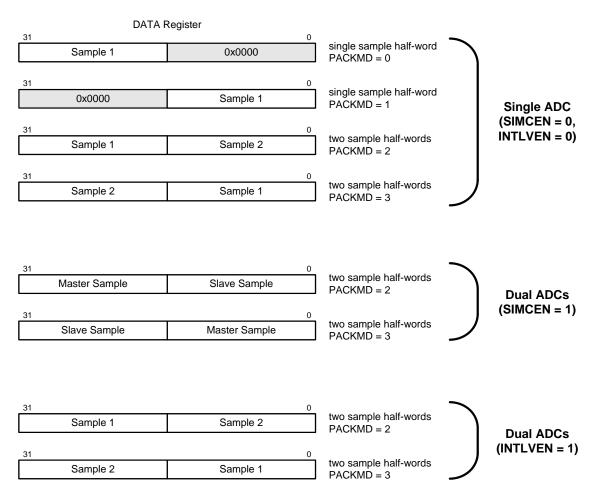
Figure 34.9. ADC Output Data Packing Options
