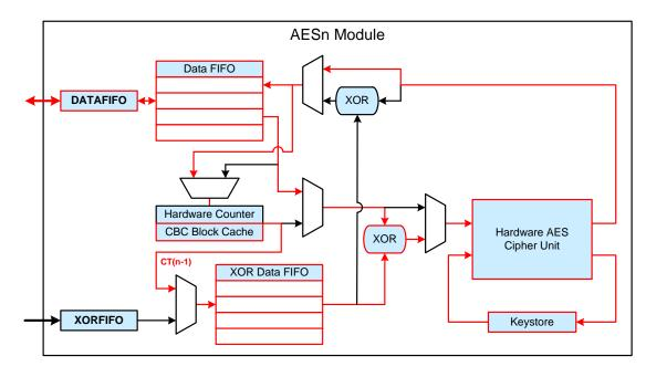
Figure 15.6. Hardware Cipher Block Chaining (CBC) AES Module Block Diagram—Encryption
