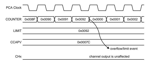
Figure 22.14. Example Software Timer Mode Timing Diagram
