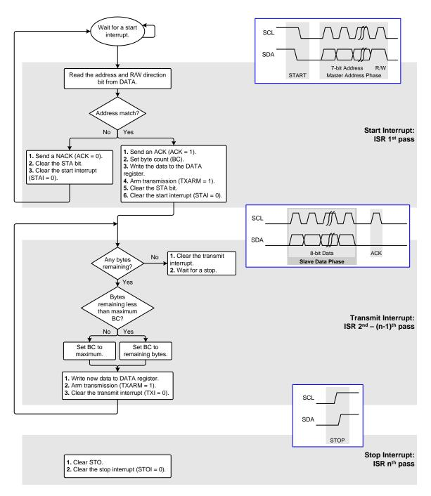
Figure 25.15. Slave Read Flow Diagram (7-bit Address)
