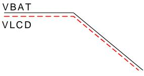
Figure 27.3. Bypass Mode
