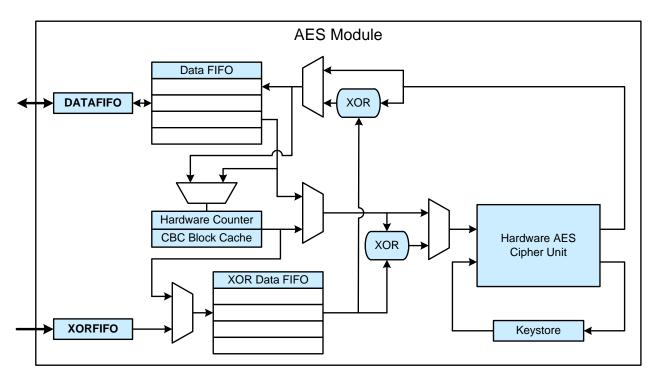
Figure 15.1. AES Block Diagram
