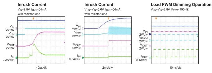
Load PWM Dimming Operation
