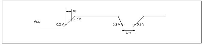
Note: Sudden change of power supply voltage may activate the power-on reset function. When changing power supply voltages during operation, raise the power smoothly by suppressing variation of voltages as shown below. When raising the power, do not use PLL clock. However, if voltage drop is 1V/s or less, use of PLL clock is allowed during operation.
