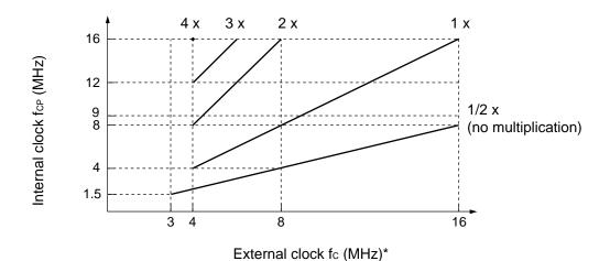
\*: fc is 8 MHz at maximum when crystal or ceramic resonator circuit is used.
