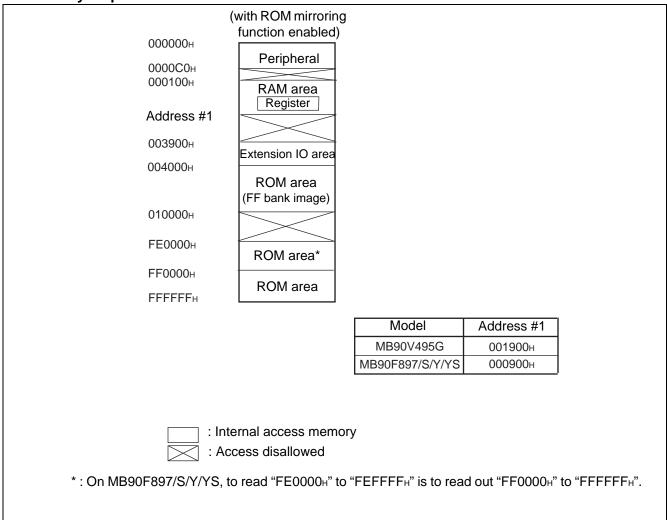
Note: When internal ROM is operating, F2MC-16LX allows viewing ROM data image on FF bank at upper-level of 00 bank. This function is called "mirroring ROM," which allows effective use of C compiler small model. F2MC-16LX assigns the same low order 16-bit address to FF bank and 00 bank, which allows referencing table in ROM without specifying "far" using pointer.
