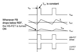
Figure 2: Heavy-Load Operation
