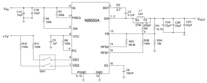
Figure 13: Typical Application with Low-ESR Ceramic Capacitor  $V_{\text{IN}}$  = 12V,  $V_{\text{OUT}}$  = 1.05/1.10/1.15/1.20V,  $I_{\text{OUT}}$  = 6A,  $f_{\text{SW}}$  = 550kHz
