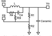
Figure 10: Simplified Ceramic Capacitor Circuit
