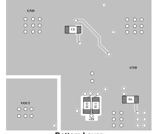
Bottom Layer Figure 16: PCB Layout Guide
