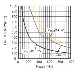
Figure 4: Plot of  $V_{\text{OUT}}$  as a Function of  $R_{\text{FREQ}}$  and the Frequency
