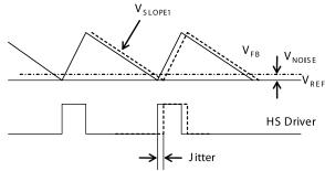
Figure 5: Jitter in PWM Mode
