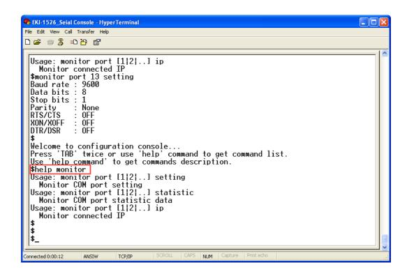
[Usage] monitor port 1|2|...|16 setting [Function] Monitor the serial ports settings
