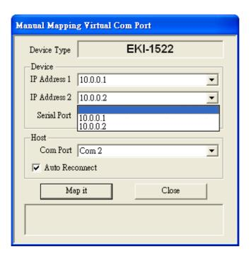
If you don't use the redundant function, just select the correct IP address in the IP address 1 field.
