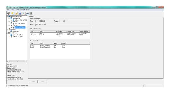
Click on the "+" before the device name, and the utility will expand the interfaces on this device server.
