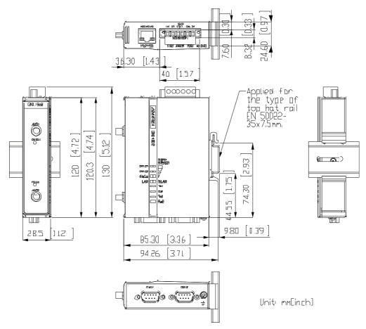
Figure 2.9 DIN-Rail Mount of EKI-1362
