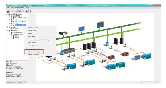
ADAM series, EDG series, and EKI wireless series have only one IP address. Select the serial port on the device server and the host COM that you want to set. Press <Map it> to establish the virtual COM port on the host.
