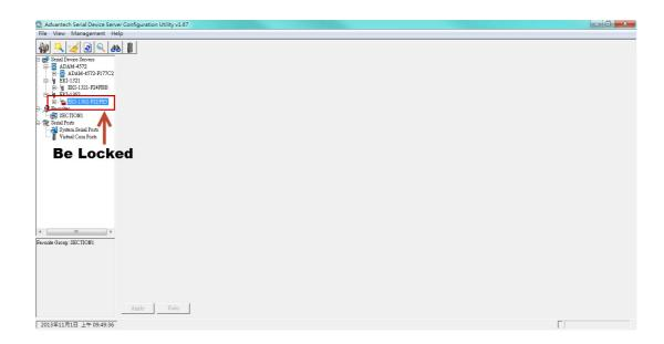
Click "Unlock Device" to unlock the serial device sever, and you need to fill in the password you have set up before. If you forgot the password, the only way to solve this problem is to restore the setting of the serial device server to the factory default which will be introduced next section.
