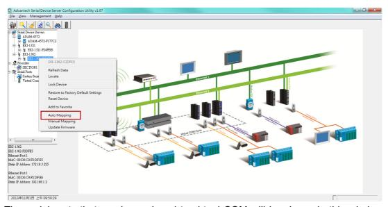
The serial ports that can be assigned to virtual COM will be shown in this window. Select the serial ports you wish to map or click the <Select All> button and press <Map Selected Ports> button. The selected serial ports will be mapped to virtual COM ports in sequential order.
