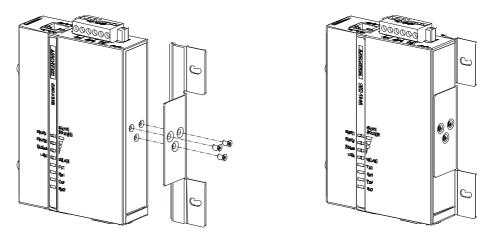
Figure 2.11 Combine the Metal Mounting Kit
