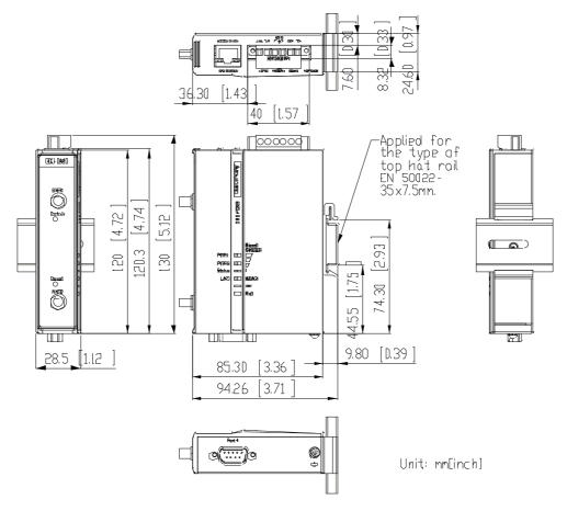
Figure 2.7 DIN-Rail Mount of EKI-1361
