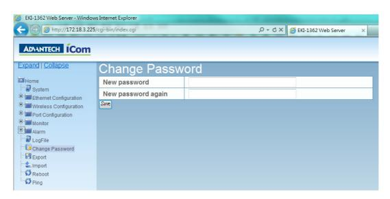
If you have set a password via the configuration utility or Telnet or serial console, when you access the web configuration, you need to key in the password. Do not need to enter the user name in the dialog.
