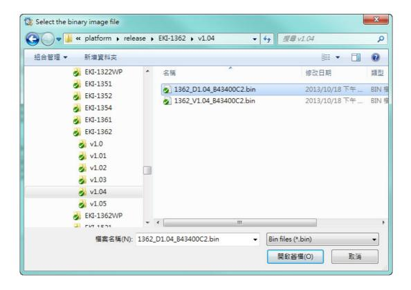
Wait for few seconds to process the updating firmware. After downloading the firmware completely, click on the "OK" button. The serial device server will restart automatically.
