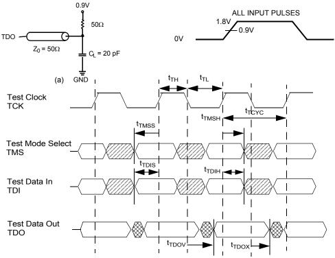
16. Test conditions are specified using the load in TAP AC Test Conditions.  $t_R/t_F = 1$  ns.
