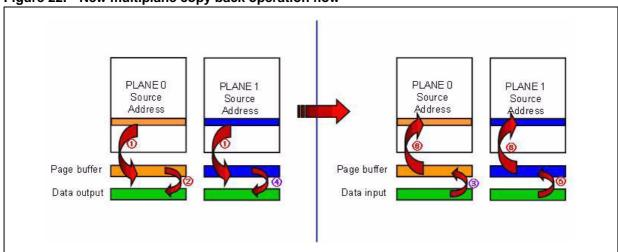
Figure 22. New multiplane copy back operation flow
