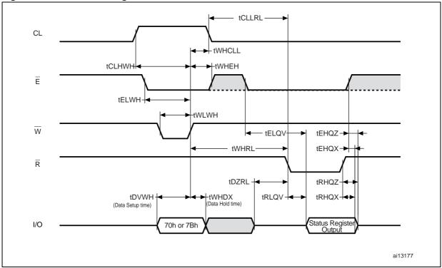
Figure 37. Read status register AC waveforms
