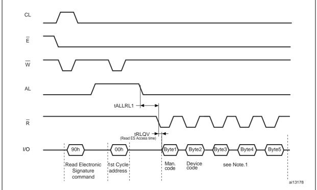
1. Refer to *Table 10* for the values of the manufacturer and device codes, and to *Table 11*, *Table 12*, and *Table 13* for the information contained in byte 3, byte 4, and byte 5.
