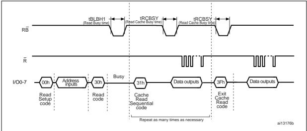
Figure 6. Cache read (sequential) operation
