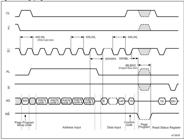
Figure 40. Page program AC waveforms
