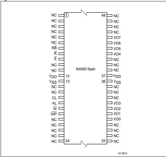
Figure 3. TSOP48 connections
