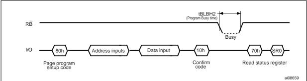
Once the program operation has started the status register can be read using the Read Status Register command. During program operations the status register only flags errors for bits set to '1' that have not been successfully programmed to '0'.
