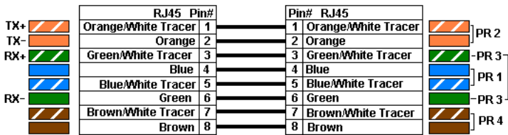
Color Standard EIA/TIA T568B Ethernet Patch Cable
