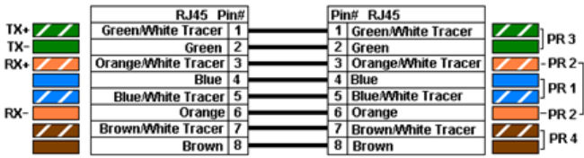
Color Standard EIA/TIA T568A Ethernet Patch Cable
