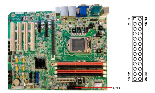
The parallel port is normally used to connect the motherboard to a printer. The AIMB-781 includes an onboard parallel port, accessed through a 25-pin flat-cable connector, LPT1.
