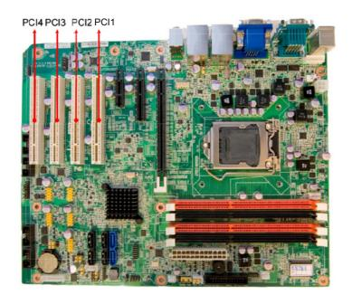
The AIMB-781 provides four 32-bit / 33 MHz PCI slots.
