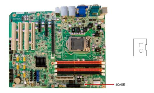
JCASE1 is for chassis with a case open sensor. The buzzer on the motherboard sounds if the case is opened.
