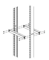
Line up shelf bracket flange holes with desired position on rack. Secure each bracket with provided #12-24 screws.
