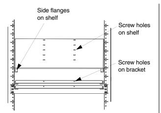
Slide side flanges of shelf through notches in brackets until screw holes line up at the desired location.
