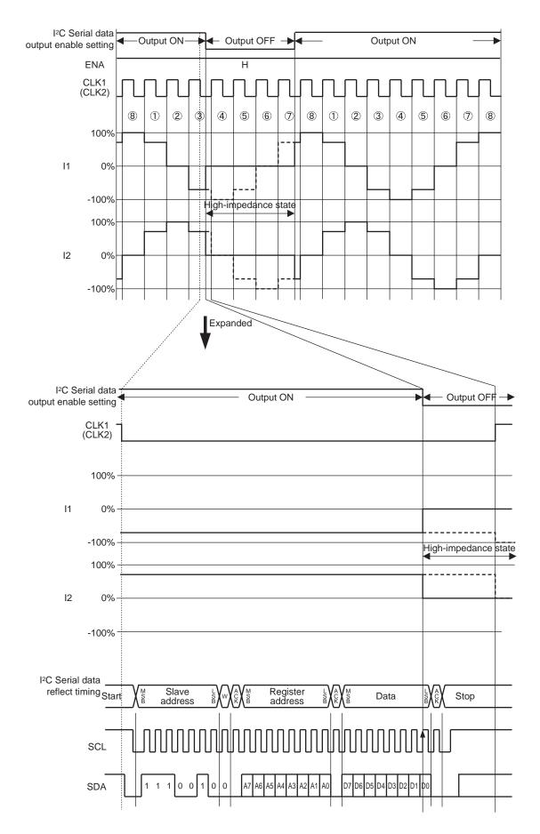
[Timing at which the output enable setting is reflected (output ON)]
