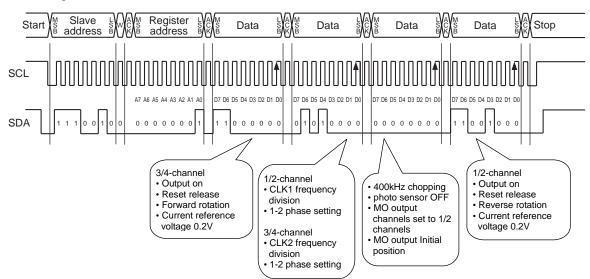
Based on the "Serial data truth table" on the next page, the following settings are used for the actual example of the continuous data transfer shown in the above figure.
