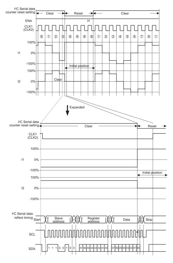
[Timing at which the counter reset setting is reflected (Reset to Clear)]
