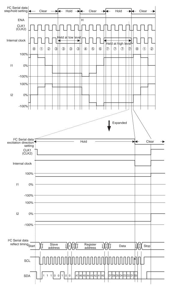
[Timing at which the step/hold setting is reflected (Hold to Clear)]
