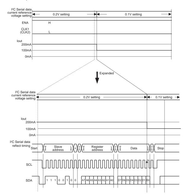
Example: With  $1.0\Omega$  for RF and 100% current ratio
