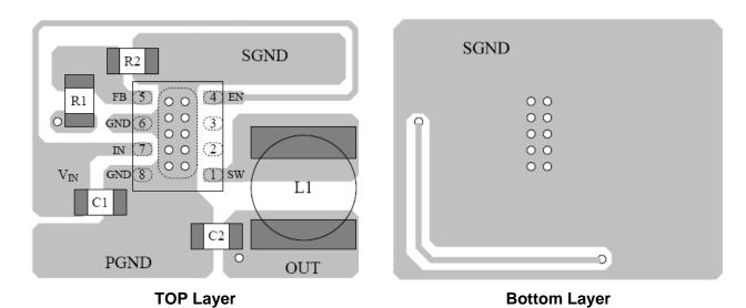
Figure 3—MP28119 Typical Application Circuit and PCB Layout Guide
