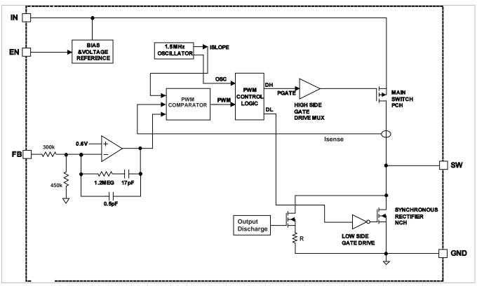
Figure 2—Functional Block Diagram (MP28119EG-1.0)
