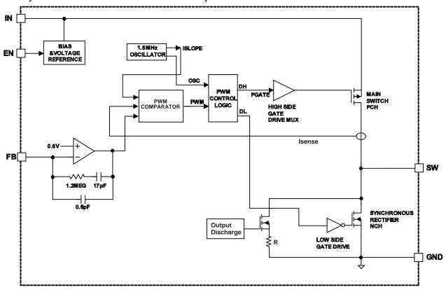
Figure 1—Functional Block Diagram (MP28119EG)
