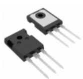
IXGH72N60C3 IGBT 600V 75A 540W TO247AD IXYS
